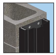
Vertical Sub Frame (Cased opening no stop) *Existing Opening Height minus 1/16"* Horizontal Sub Frame (Cased opening no stop) *Existing Opening Width minus 3 3/16"* Vertical Finished frame dimension *Existing Opening Height minus 2"* Horizontal Finished frame (header) *Existing Opening Width minus 4"*
