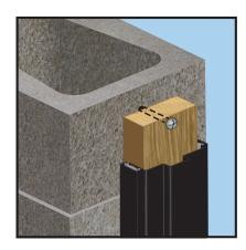
Vertical Sub Frame – wood, ripped to standard frame width *Existing Opening Height minus 1/16"* Horizontal Sub Frame - wood, ripped to standard frame width *Existing Opening Width minus 3 1/16"* Vertical Finished frame dimension *Existing Opening Height minus 2"* Horizontal Finished frame (header) *Existing Opening Width minus 4"*
