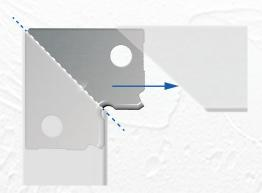
MiterGard is factory-attached to vertical casing. Exposed section slides securely into header casing
