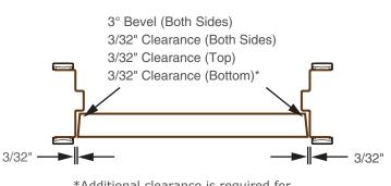
\*Additional clearance is required for Thresholds and various floor conditions.
