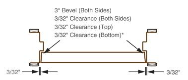
\*Additional clearance is required for Thresholds and various floor conditions.
