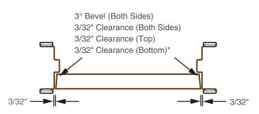
\*Additional clearance is required for Thresholds and various floor conditions.
