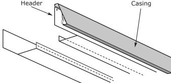
When all casing pieces are aligned, snap the header casing over
