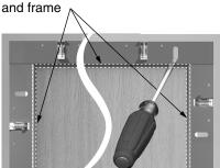
5. Hang the door. To align the frame and door, first close the door. Then begin with the header, using a screwdriver inserted in the alignment slot closest to the strike jamb. Create an equal gap between door and frame, and fasten the header above the strike jamb and the remainder of the header at every clip on the door side only.
