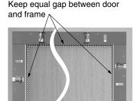
Fasten the header above the strike jamb and the remainder of the header at every clip on the door side only.
