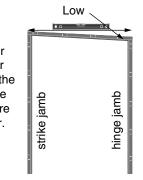
If the level indicates that the hinge jamb is lower than the strike jamb, lift the header until it is level and fasten one screw in the header over the hinge jamb. Lift the hinge jamb tight to the header. Align the corner of the hinge jamb with the corner of the header and fasten at an upward angle at the top of the hinge jamb to ensure that the hinge jamb is snug to the header. On the opposite side of the hinge jamb, repeat the above steps when attaching the closure pieces.
